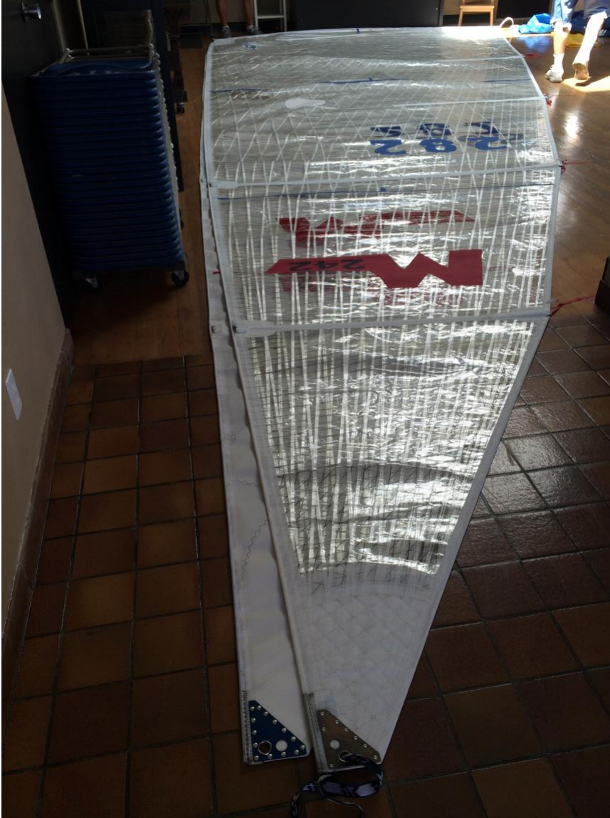
The North sail also has about 6 more inches of foot material than the UK sail.
