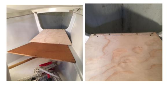
2. Interior motor mount. Self-explanatory, and requires the purchase of a 2<sup>nd</sup> mount. Also requires a nice rectangular hole cut in the cross-board, with support wood pieces screwed in underneath on each side so that the cut-out piece can be put back in place if you go cruising in the 242 and want to put cushions up forward. The motor would of course be put on the transom mount at this point.
