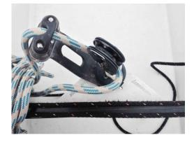
Lastly, with regard to the center post system, I inserted this "tie-down" system at the suggestion of Jason Rhodes so the possibility of the center post system twisting under load was greatly reduced or eliminated. All that is required is an eye-bolt through the
