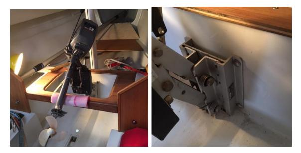
3. The battery case is best moved from the back storage area under the cockpit and placed at the aft end of the cabin sole for easy access, which is Class legal. I tied mine in place with 2 eyestraps that are just screwed in (not bolted in because of the hassle factor). My battery weighs 37 pounds, so the aft Corrector Weights include the 8 pound top-up
