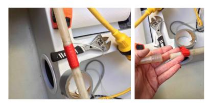
Above: you can see how a double-sided hose barb is inserted in a cut in the drain hose. In this manner the whole dehumidifier setup can be removed from the boat while racing, and all you are left with inside the boat is the aft end of the drain hose (below). It's a pretty slick setup, per the next photo:
