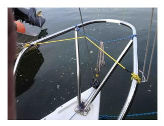
Note in the photo below that the furling drum rope is wound counter-clockwise (the opposite of what this old photo above shows): this helps with the jib furling at the weather mark because the tack-board of the sail begins to roll easier in the counter-clockwise direction, so friction is greatly reduced. If you furl clockwise, as shown in the above photo, the tack-board rubs hard against the stanchion causing excess friction.
