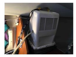
The dehumidifier then sits on top of the board in its Styrofoam shipping base for stability. Note that there are two very long sail ties attached to the handle of the dehumidifier so it can easily be lowered down to ground level by one person, or lifted up again by a single person when it is being re-inserted into position in the boat post-racing.
