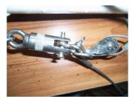
If the inside edge bearing surface is worn excessively, you can replace the fitting with a small Harken swivel #164 (standard load version):
