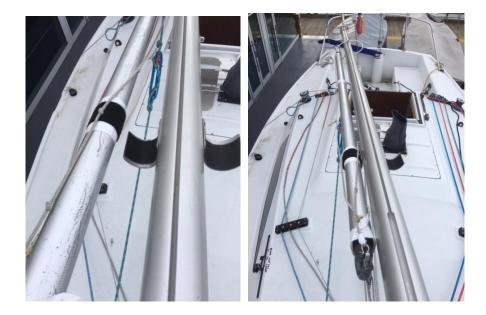
12. Does the boat have tweakers for extremely windy conditions? There are two advantages: a) they can be used to choke the chute in very windy conditions and depower it as well as stabilize it, and b) the pulling points on the boat are moved forward by 10 feet so you are less likely to do a banana-split broach in heavy air.
