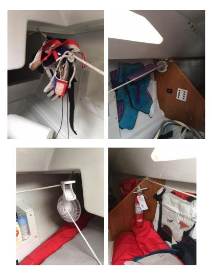
The fan clipped on the aft starboard line is particularly useful for circulating warm air into the aft end during the winter months, which otherwise would be a moist cold air trap zone. The heater in the photo below is essential, and I put an old piece of tin foil under it just in case of an electrical malfunction:
