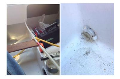
Above: a zap-strap holds the hose in place at the cockpit side of the hole drilled for the drainage hose.
