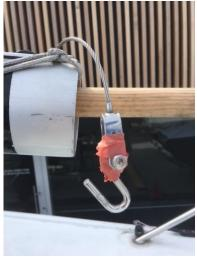
18. And because there is always the possibility of the outhaul wire breaking or the mainsheet fitting pulling out of the boom, I have backup lines ready to go in both cases, per the following two photos.
