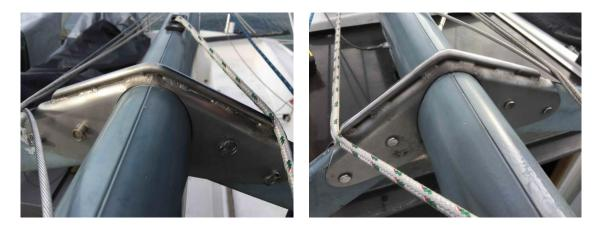
5. Check that the upper furler fitting is not wearing thru on its upper inside edge where it connects to the mast lug-hole via a shackle. Shown below is a sample very old fitting:
