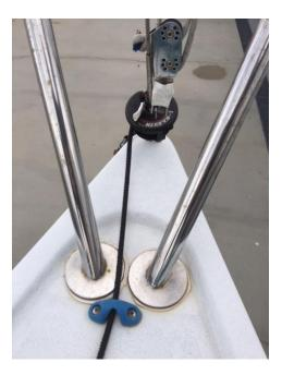
14. On my old boat it came with a small Harken block just behind the furling drum to help guide the furling line. In the photo above it's a plastic eyestrap with a metal insert to reduce friction:
