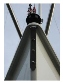
11. Buy four 6' long or so white shroud covers so that the boom rubs against them and not the shrouds. They are about \$3 each. Also tape a short batten (12") on each side of the boom so that it is also interspersed between the boom and the shroud covers.
