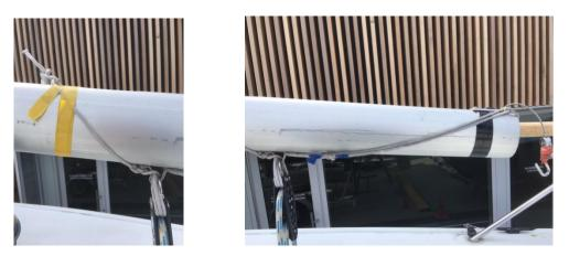
19. The topping lift loves to jam between the top of the lower shrouds and the mast, so tying a piece of thin string across the front of the mast, per the photo, is a must-do. And per the  $2^{nd}$  photo, this can be accomplished by placing ladder feet on a wet towel on the deck, and tying the ladder 4 different ways at the base and also up high 3 different ways so it cannot move.
