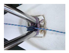
15. Everyone has different jib downhaul assemblies – this is mine on my old boat, 171, which is the same one on my new boat that connects to a horizontal tang on top of the furling drum:
