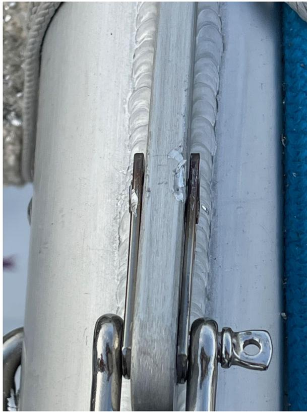
A top-down view with the cross-bolt inserted, plus washers. What you don't see is the end of the bolt: we broke it off with pliers in line with the top of the lock-nut via wiggling the bolt up and down a few times.
