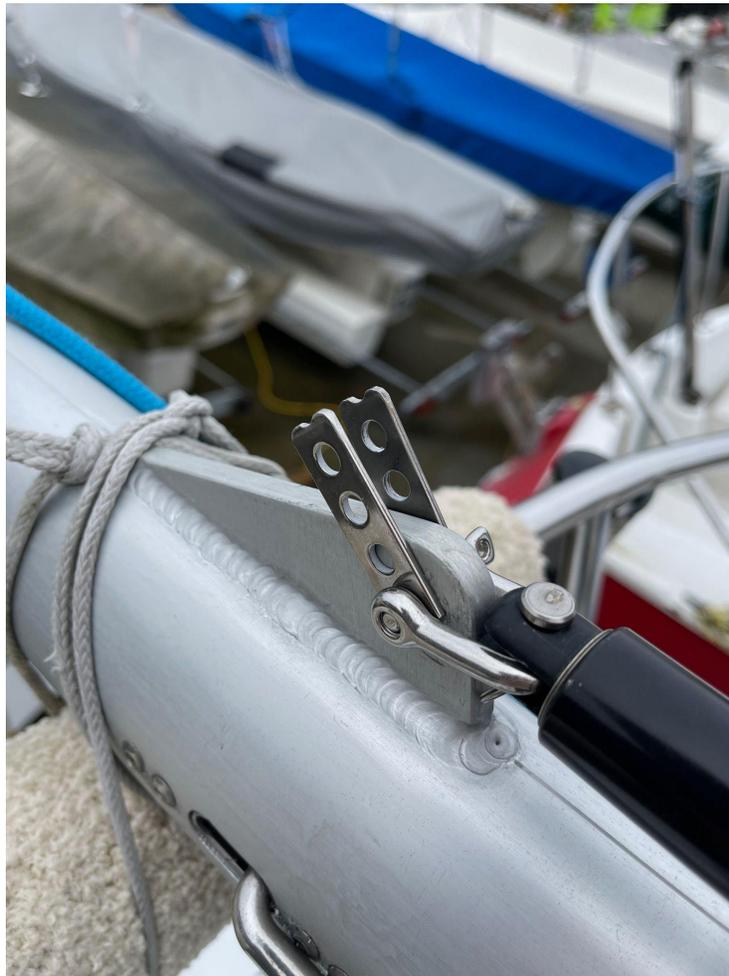
Then fully-assemble the lower section and drill a smaller pilot hole higher up. Once it is drilled then you can use a larger bit to enlarge the Upper Assembly hole so it will accommodate the upper bushing.
