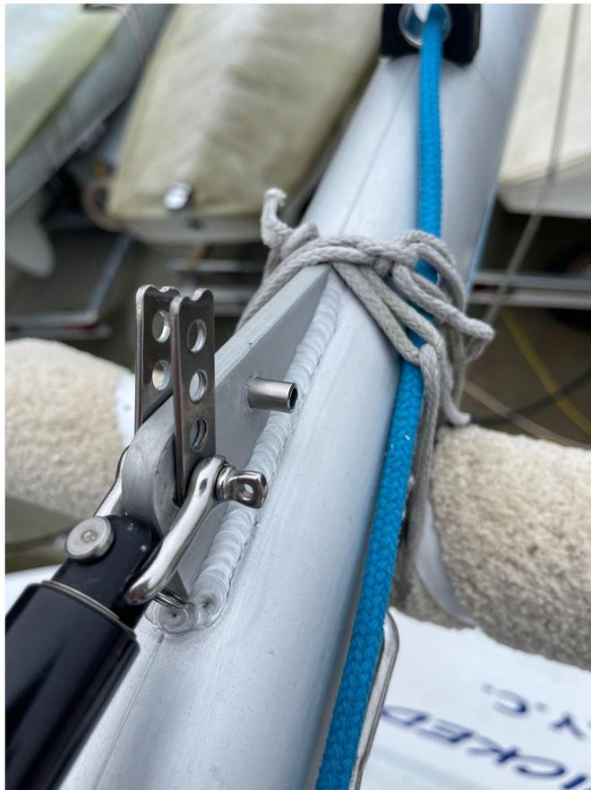
Then we used the larger drill bit on the tangs so they could also accommodate the larger bushing. This took quite a while. Then we used the Dremel to burn off the metal burrs on the tangs.
