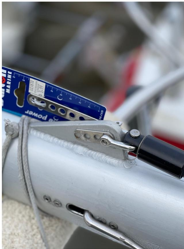
Use a handheld drill to enlarge the lower hole to accommodate the new stainless bushing, and then do a dry fit of that bushing, per the 2nd photo.
